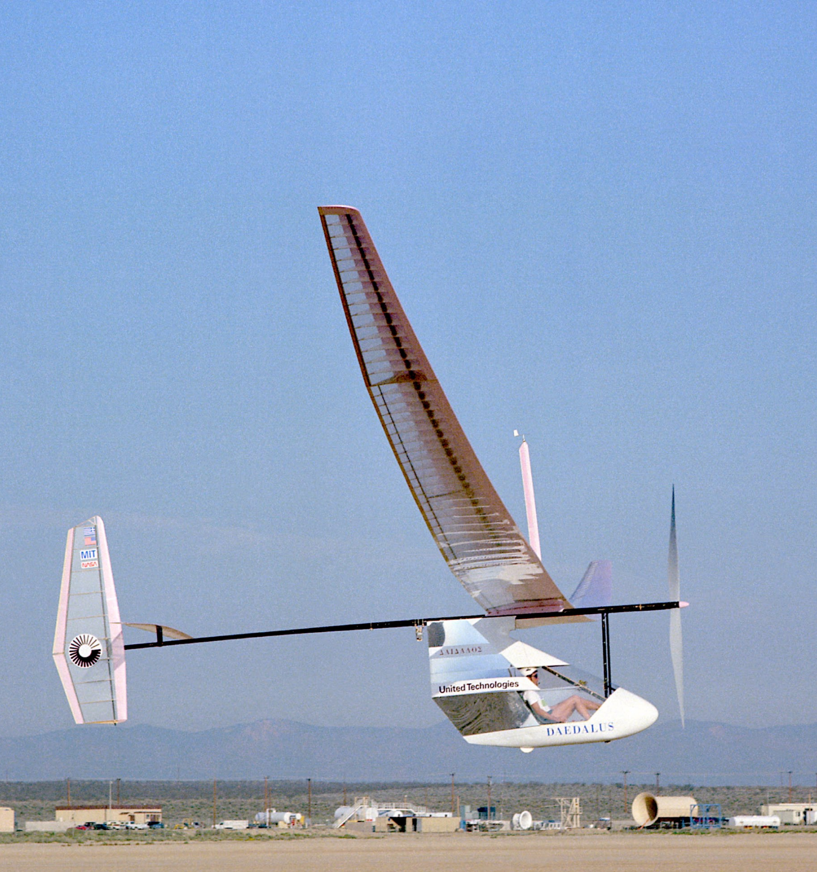
THE DAEDALUS HPA, CONSTRUCTED BY STUDENTS AND STAFF AT M.I.T. AND FLOWN ACROSS THE AEGEAN SEA IN 1988.
