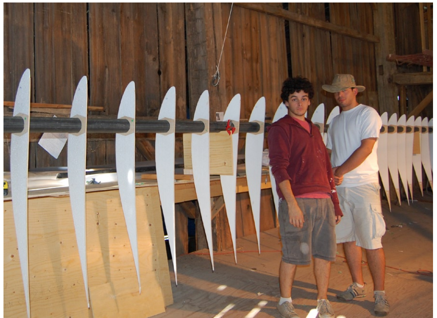
HPO LEFT WING AFTER COMPLETED RIB ASSEMBLY (ABOVE)
